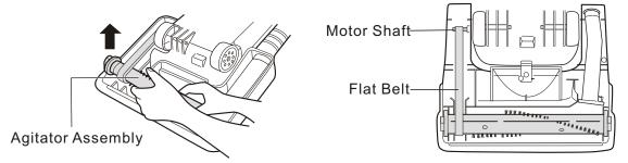
3 Place a new flat belt onto the motor shaft and pulley.
